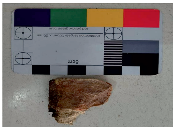
Fig. 7: Shows a lime mortar sample from Curdi.
